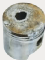
A damaged piston
